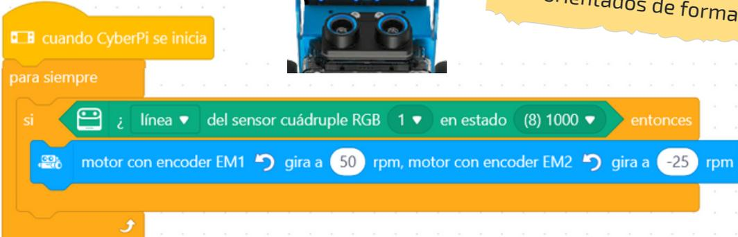
The image shows a Scratch code block for a line-following robot. It starts with a 'when CyberPi starts' event block. This is followed by a 'forever' loop block. Inside the loop, there is a conditional block: 'if line sensor 1 is at 1000, then'. The 'then' block contains two motor control blocks: 'motor with encoder EM1 turns at 50 rpm' and 'motor with encoder EM2 turns at -25 rpm'. The robot is shown in the background with labels L2, L1, R1, and R2 for its sensors.
