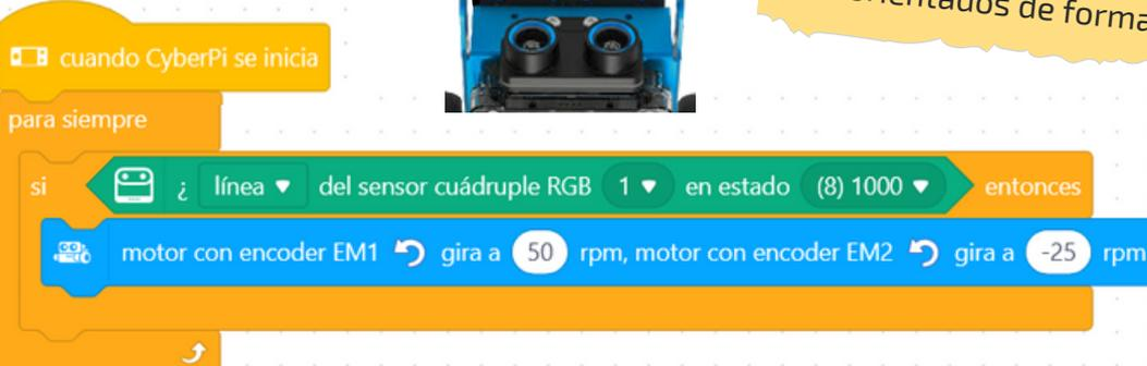
The image shows a Scratch script for controlling the mBot. The script starts with a 'when CyberPi starts' block, followed by a 'forever loop' block. Inside the loop, there is a 'if' block that checks if 'line' of the 'RGB quadruple sensor' is in state '(8) 1000'. If true, it triggers two 'motor with encoder' blocks: 'motor with encoder EM1' set to '50 rpm' and 'motor with encoder EM2' set to '-25 rpm'. The motor labels EM1 and EM2 are highlighted in blue in the original image.
